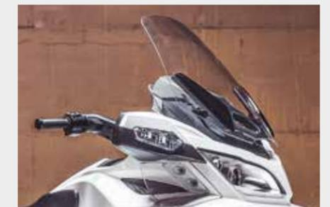
**ADJUSTABLE ELECTRIC WINDSHIELD:** Wide range of wind protection and adjustable with the push of a button.
